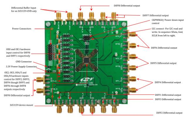
**Figure 1. Evaluation Module Front Panel**
