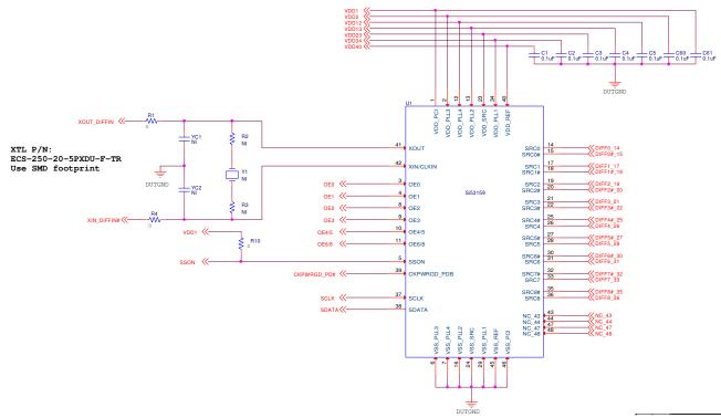
Figure 2. QFN-48 Device Connection
