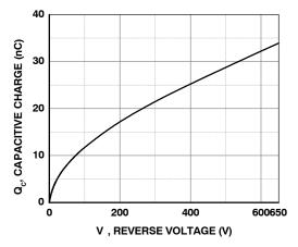
Figure 6. Capacitive Charge vs. Reverse Voltage
