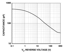
Figure 7. Capacitance vs. Reverse Voltage
