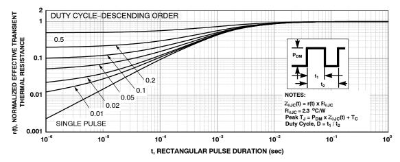
Figure 9. Junction-to-Case Transient Thermal Response Curve
