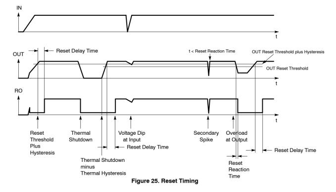
During power-up (or restoring OUT voltage from a reset event), the OUT voltage must be maintained above the Reset threshold for the Reset Delay time before RO goes high. The time for Reset Delay is determined by the choice of IC and the state of the DT pin.
