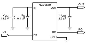
Figure 1. Application Diagram
