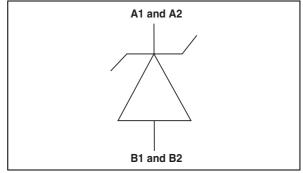
Note: B1 and B2 bumps must be grounded on the PCB together
