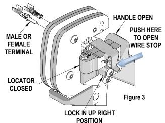
To raise the wire stop, press the tab on the wire stop as shown in Figure 3. Insert the proper terminal into the
