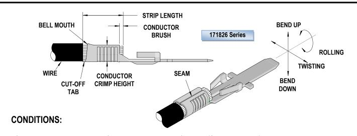
After crimping, the conductor profiles should measure the following (See notes below).
