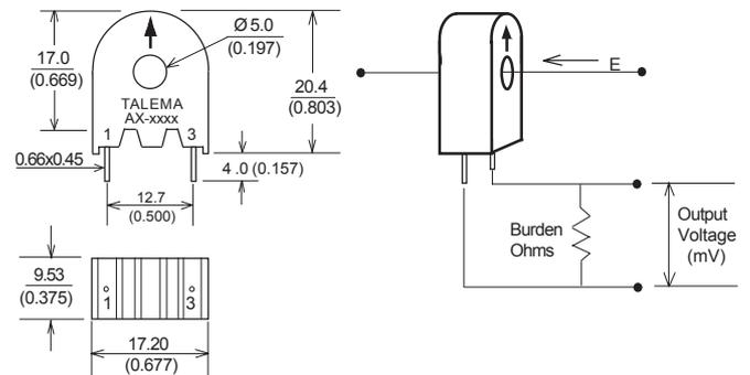
Dimensions are in mm. General Tolerance  $\pm 0.25\text{mm}$  unless specified.
